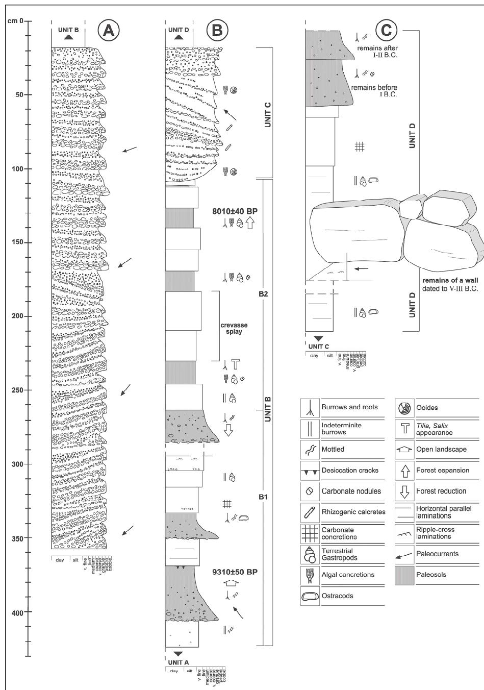
Fig. 2 - Stratigraphic section studied in the Corso del Popolo site of the Terni basin. The different units are described in text. A: Unit A, related to coarse-grained point bar deposits; B: Unit B, an overbank sequence formed of levee (B1) and crevasse-splay (B2) sediments interbedded with floodplain deposits; C: Unit C, a crevasse channel deposit; D: Unit D, sequence due to a cut-off event.
