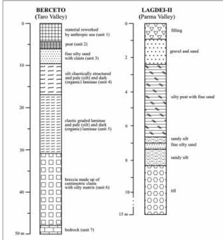
Figure 2 - Lithological features of Berceto and Lagdei-II boreholes.
