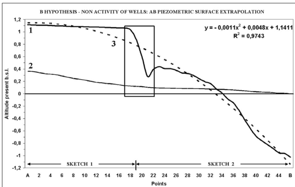
Fig. 6b - Real hydrogeological section and theoretical best - fitted on 2<sup>o</sup> degree equation extrapolation for **B** scenario. The rectangle represents the present Archaeological Park area. 1 = Past Piezometric Level; 2 = Present Piezometric Level; 3 = Past Extrapolation Level based on "Y" 2<sup>o</sup> degree equation.
