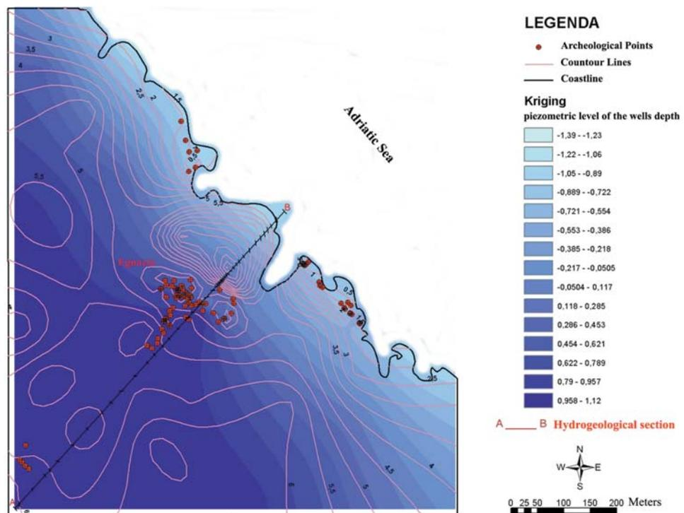
Fig. 5 - Piezometric surface restitution of Egnazia town, by means of ArcMap 8.3 GIS software, for **B** scenario.
