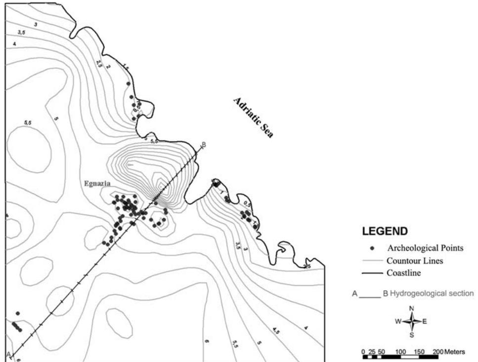
Fig. 4 - Topography restitution of Egnazia town, by means of Surfer 8 software, with contour lines. ⊗: Archaeological Points; —: Contour Lines; —: Coastline; AB: Hydrogeological section track.
