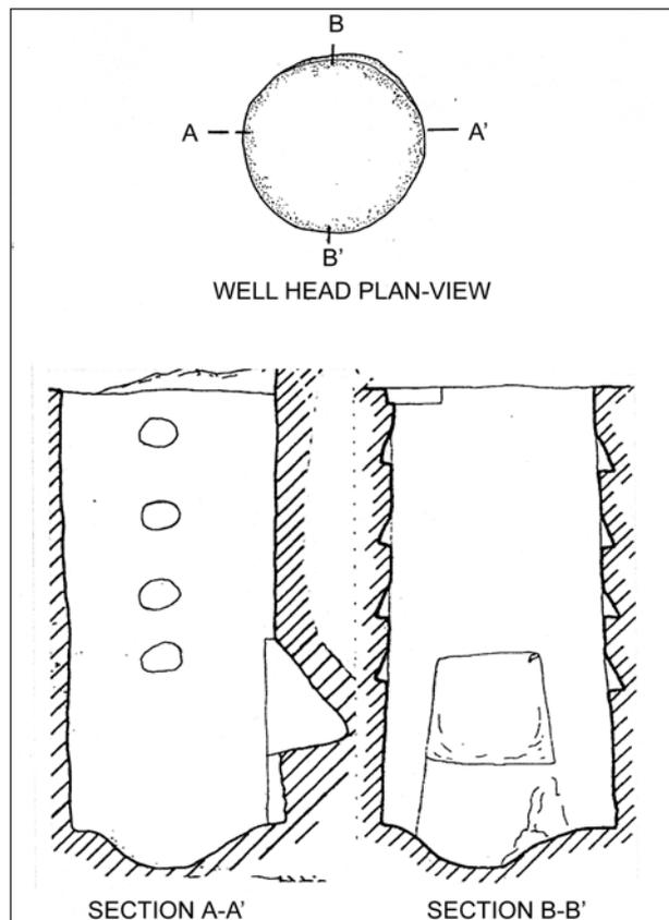
Fig. 3 - Well Scheme: in the vertical sections 4 cavity for each side, named "pedarole", can be distinguished. In the lower part a vertical sub-rectangular cavity opens (from Digging Journals).
