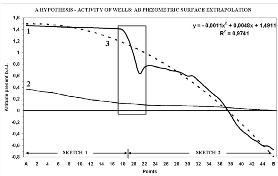
Fig. 6a - Real hydrogeological section and theoretical best - fitted on 2<sup>o</sup> degree equation extrapolation for **A** scenario. The rectangle represents the present Archaeological Park area. 1 = Past Piezometric Level; 2 = Present Piezometric Level; 3 = Past Extrapolation Level based on "Y" 2<sup>o</sup> degree equation.
