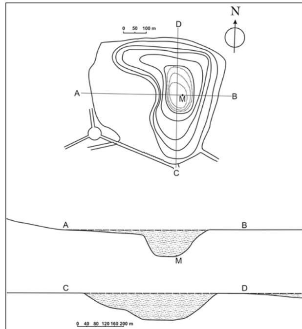
Fig. 3 - Pantano Piccolo salt marsh: above, map of the isobaths (continuous curve distance 5 m and dot curves distance 1 m, maximum depth  $M = -28$  m); below, altimetric-bathymetric profiles along A-B and C-D shares (derived from ABBRUZZESE & GENOVESE, 1952).
