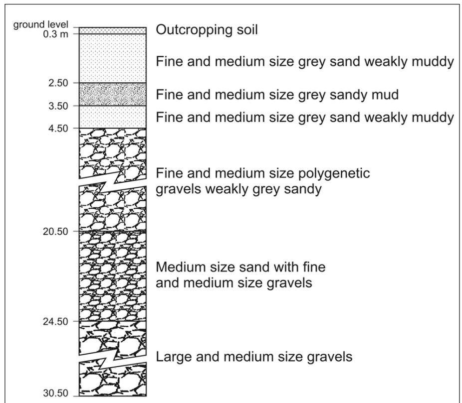
Fig. 9 - Shallow stratigraphy resulting from geognostic boring 300 m at W of La Torretta (D<sub>2</sub>, in Fig. 2).
