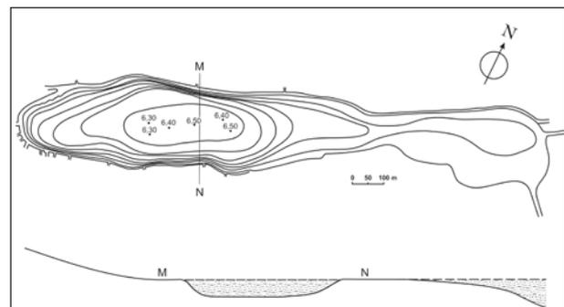
Fig. 4 - Pantano Grande salt marsh: above, map of the isobaths (continuous curve distance 1 m); below, altimetric-bathymetric profile along M-N share.
