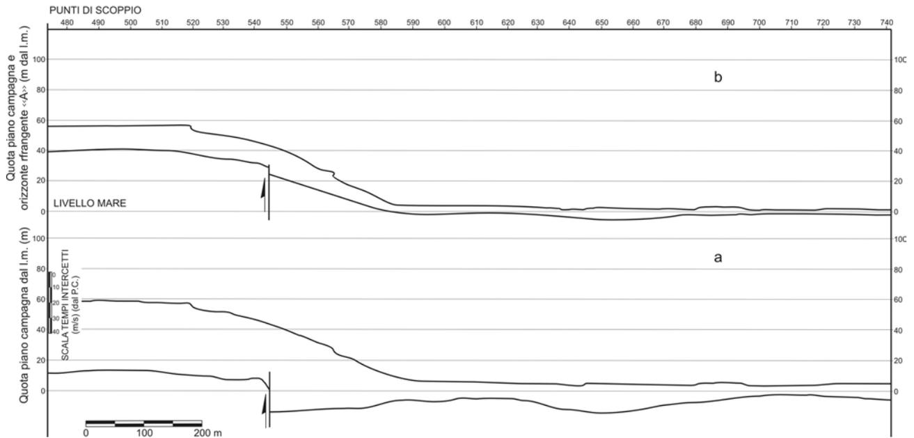
Fig. 6 - SM-7 seismic high resolution profile along E-F share (Fig. 1): a) diagram of the intercept-times; b) seismic section (after DEL BEN & FINETTI, 1985).
