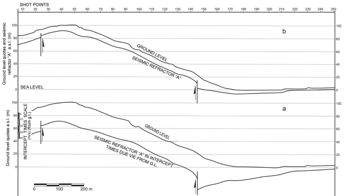
Fig. 5 - SM-2 seismic high resolution profile along C-D share (Fig. 1): a) diagram of the intercept-times; b) seismic section (after DEL BEN & FINETTI, 1985).
