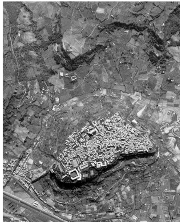
Fig. 6 - Aerial photograph of the Orvieto area. Mass movements can be observed along the slopes. (Region of Umbria; scale: 1:33,000; photo date September - October 1977; SMA permission no. 38: 01/02/1978 execution. Photo by: Compagnia Generale Riprese aeree - Parma).
