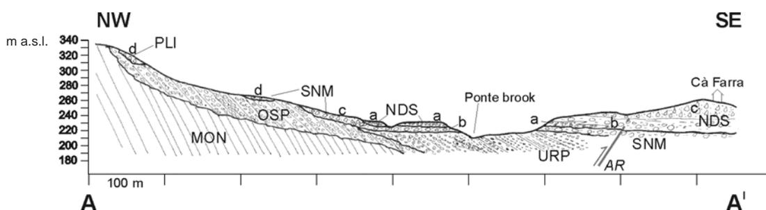
Fig. 2 - Schematic cross section of Rio Ponte section (A-A' in Fig. 1). MON: Montello Conglomerate; OSP: Osoppo Conglomerate; URP: Rio Ponte Unit; PLI: Plaino Synthem; SNM: Santa Margherita Synthem; NDS: Canodusso Synthem; a: alluvial deposits; b: lodgment till; c: ablation till; d: "loose skeletal till"; AR: Arba-Ragogna thrust.
