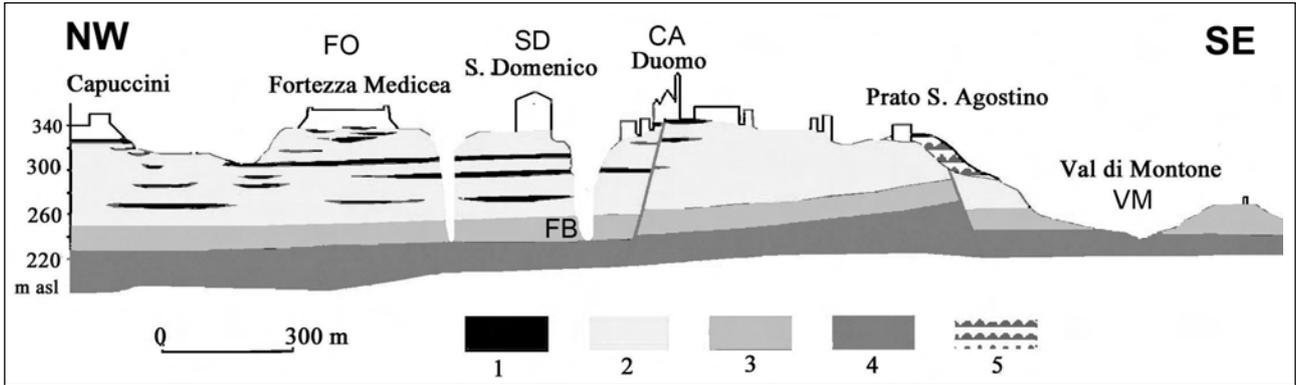
Fig. 2 - Schematic cross-section of the Pliocene deposits under Siena (1: marine silty clay; 2: sandstone; 3: basal argillaceous sandstone; 4: sandy conglomerate lenses; straight inclined line below the Cathedral (Duomo): normal fault; CA: Duomo (Cathedral); FB: Fontebranda; FO: Fortezza (Fort); SD: S. Domenico; VM: Val di Montone; see location of cross-section on Figure 3). (After LAZZAROTTO & PASCUCI, 1998).
