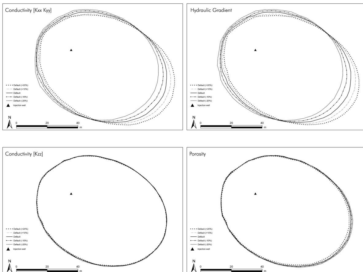
Fig. 10 - Location of 16.0°C isotherms after 60 days of injecting warmer water for various values of Horizontal and vertical conductivity, hydraulic gradient and porosity.
