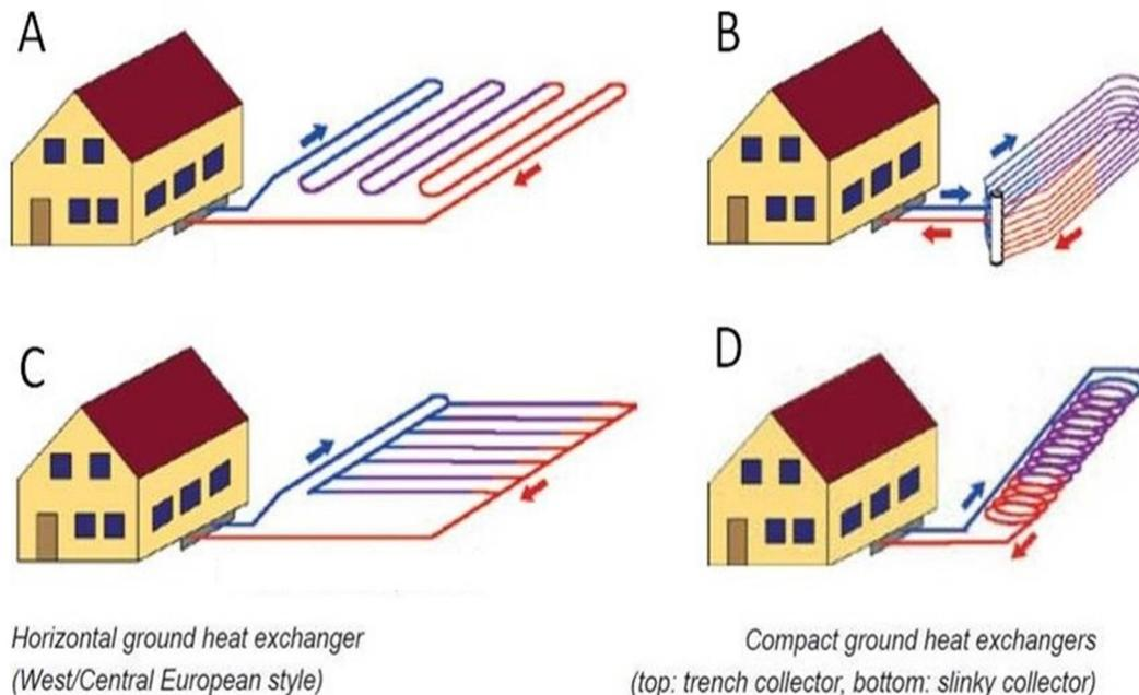
Fig. 1 - Closed-loop horizontally system, with ground source heat pump (GSHP). Various type of configuration are represented: A) connection in series, B) trench connection, C) connection in parallel and D) spiral slinky connection (Rafferty, 2000; Lund, 2007).
