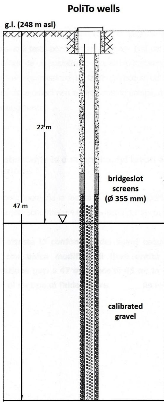
Fig. 6 - Technical scheme of the Politecnico wells, utilized for Open Loop System (GWHP).
