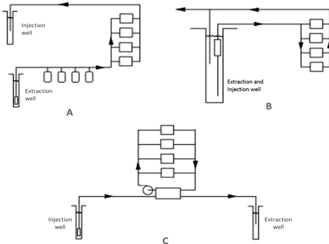
Fig. 4 - Several types of Open-Loop Systems: A) Direct open loop heat pumps; B) Standing Column Systems (SCW); C) Indirect Open Loop Systems (Rafferty, 2001).
