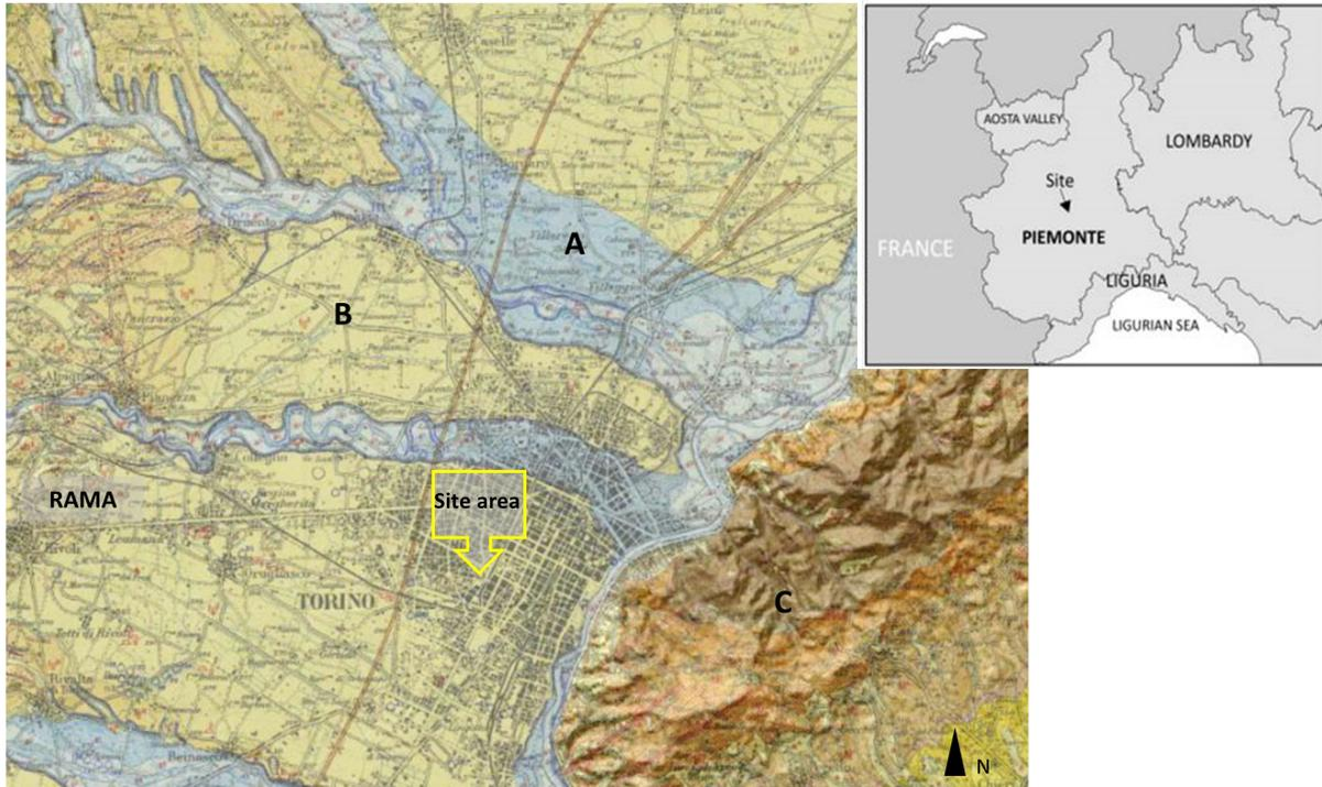
Fig. 8 - Geological sketch map, with the main geological Units that represent the Turin area. (Geological Map of Italy, scale 1:100000, layout 56, not in scale) where **A**: Unit 3, fluvial deposits; **B**: Unit 3, Fluvio-glacial deposits; **C**: Unit 1 and Unit 2, Tertiary Succession; **RAMA**: Rivoli-Avigliana Morainic Amphitheatre.
