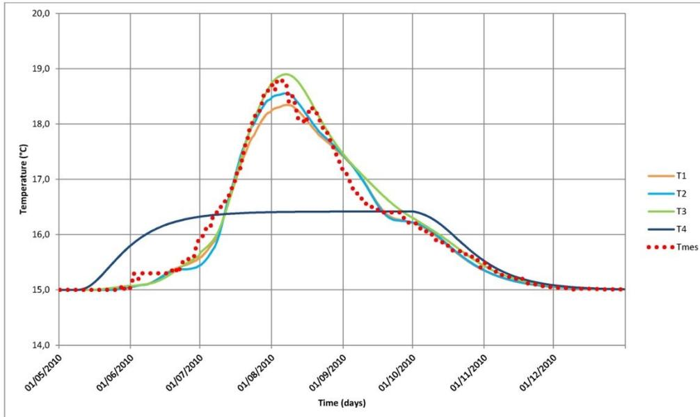
Fig. 11 - Temperatures in piezometer S2. The dotted line corresponds to the measured data
