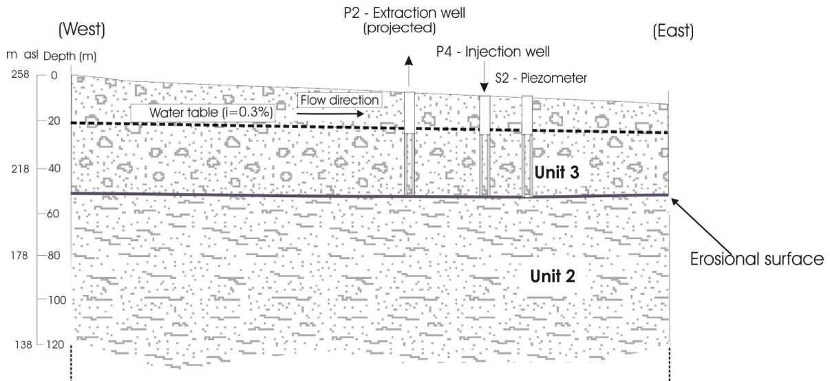
Fig. 9 - Cross-section of the Open Loop System (GWHP) installed in the "Politecnico di Torino" for cooling some of the university buildings.
