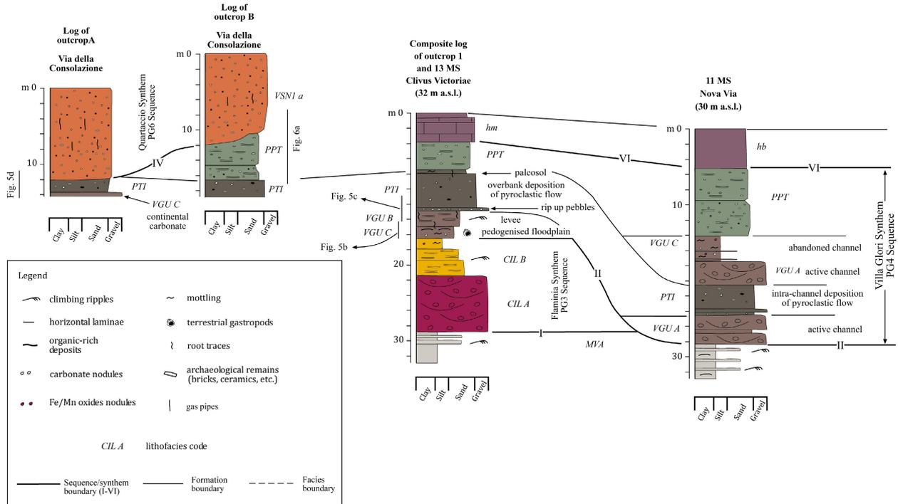
Fig. 7 - Correlated sedimentary logs from selected boreholes and key outcrops along the Velabro Valley and in the north-western Palatine (see Fig. 2b for location).
