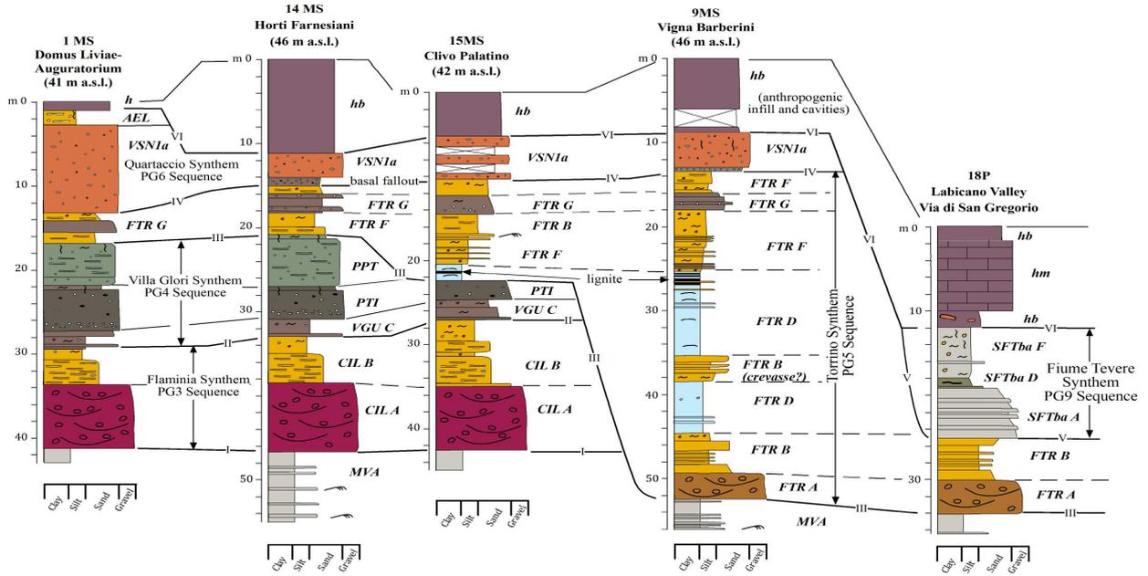
Fig. 8 - Correlated sedimentary logs from selected boreholes from central Palatine Hill (see Fig. 2b for location). Legend as in Fig. 7.
