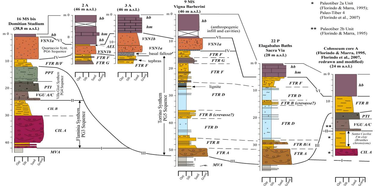
Fig. 9 - Correlated sedimentary logs from selected boreholes in the eastern Palatine Hill and Oppius Hill (see Fig. 2b). Note the internal facies variability of the Fosso del Torrino Formation (FTR) reflecting intercalation of crevasse sandy deposits within floodplain muds. Legend as in Fig. 7.
