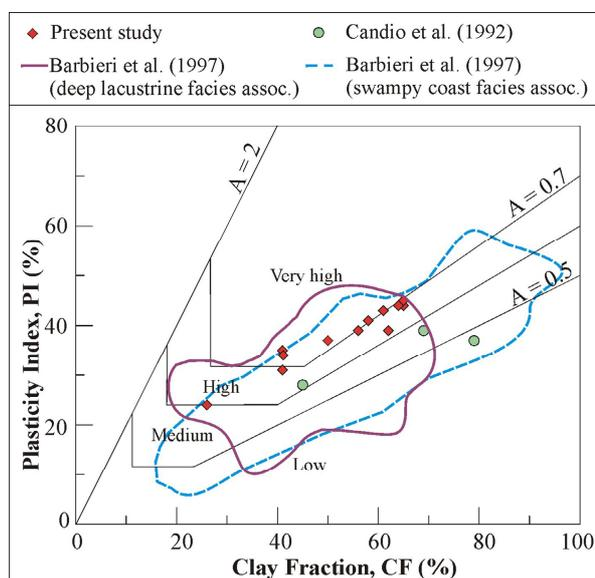
Fig. 7 - Skempton's activity chart (modified after Williams & Donaldson, 1980) for soils in Table 1 and those from Candio et al. (1992). Data from Barbieri et al. (1997) were elaborated from original graph (only boundaries of data were represented).
