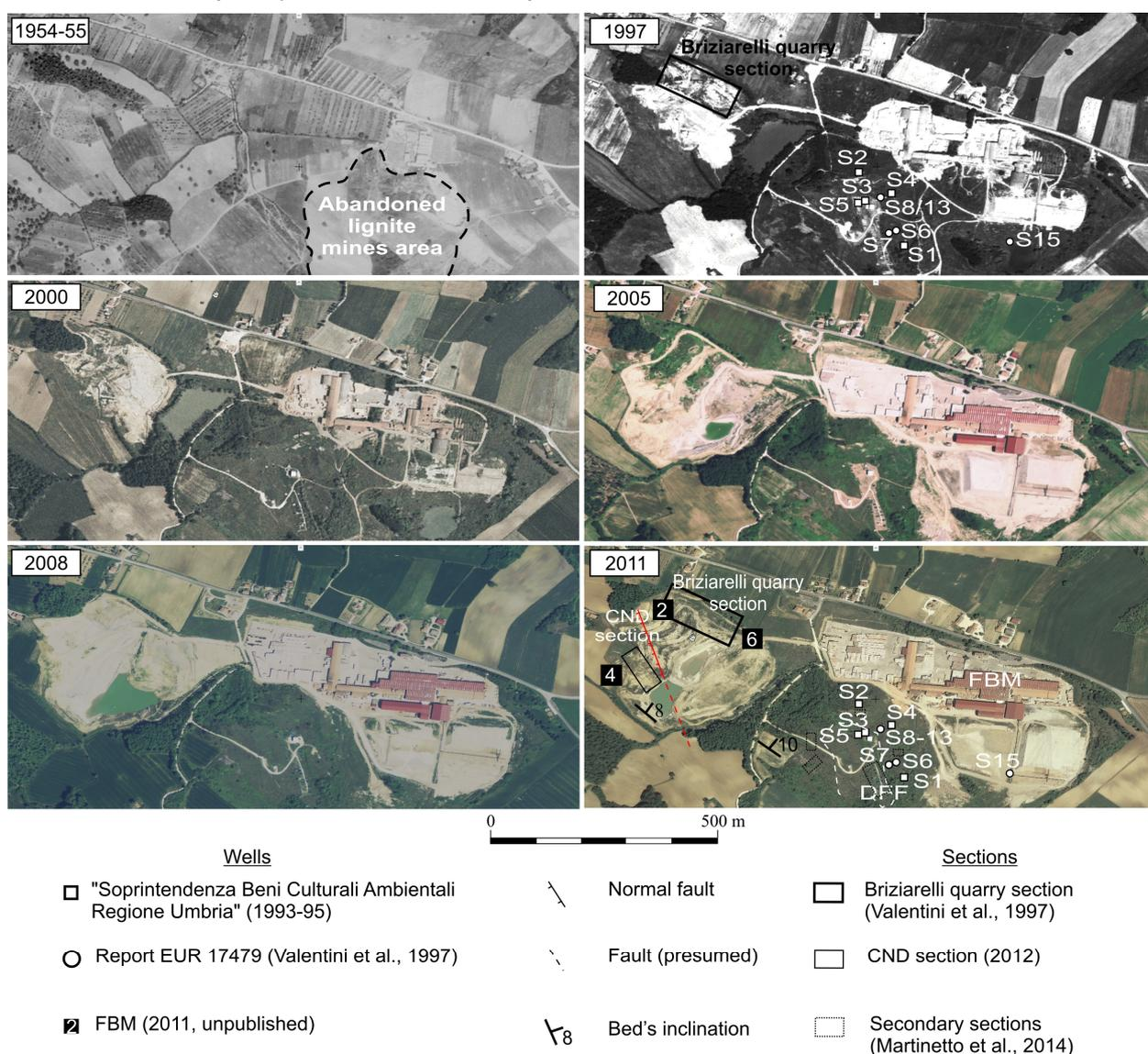
Fig. 2 - Evolution of the Cava Nuova quarrying area (CND) and of the Dunarobba Fossil Forest area (DFF) through time. Positions of stratigraphic sections and wells are reported.
