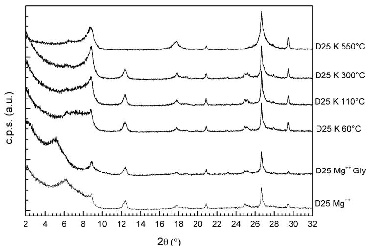
Fig. 8 - XRD patterns collected on oriented mounts of CND25 sample, saturated with Mg<sup>++</sup> and K<sup>+</sup>, as example.
