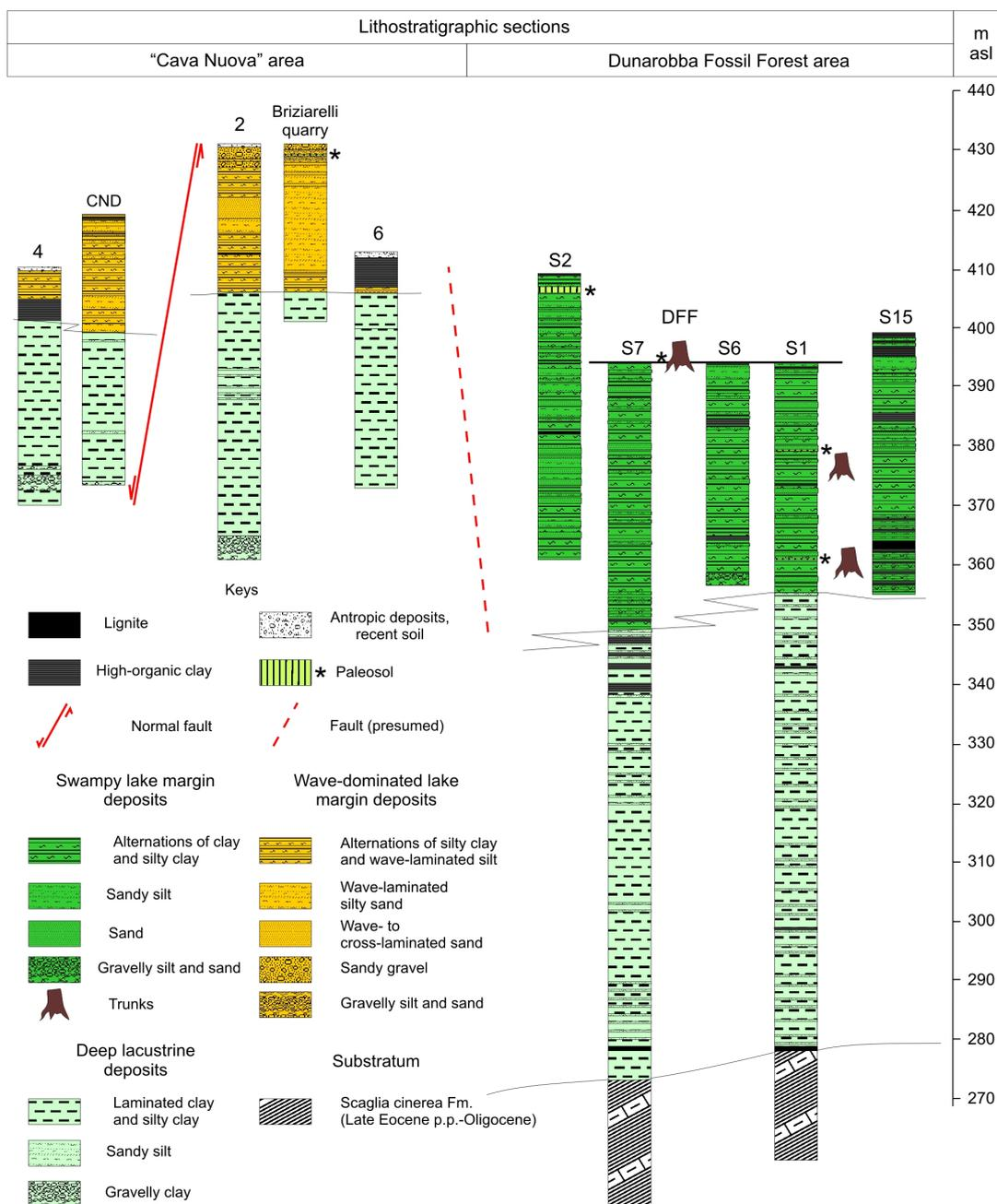
Fig. 5 - Comparison of selected lithostratigraphic columns in the Dunarobba area from recent and further data.
