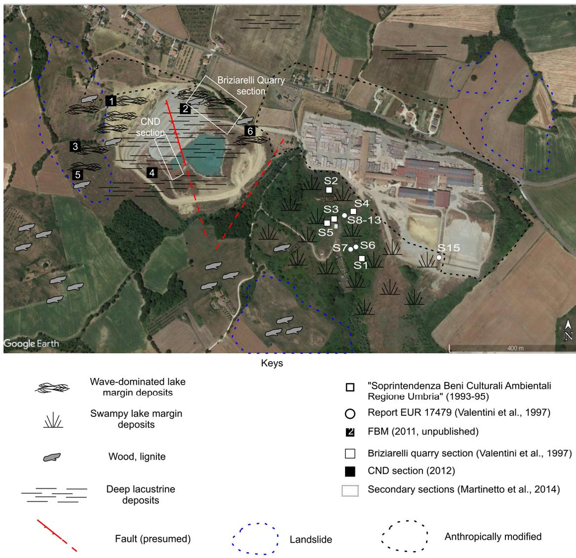
Fig. 6 - Schematic distribution of facies across the Cava Nuova and the Fossil Forest areas. Landslide and anthropically-modified sectors are also perimtered.
